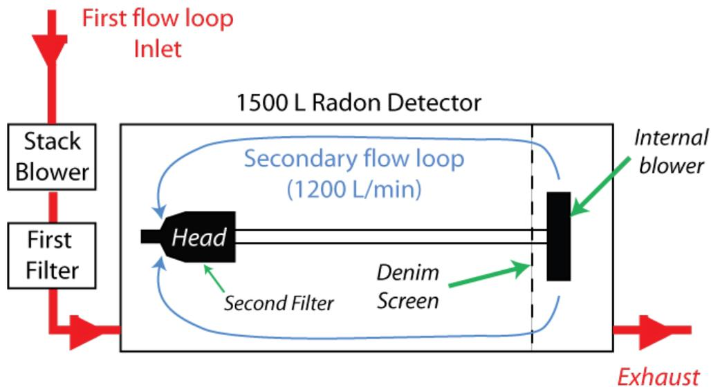
*Figure 11: Schematic of the internal and external flow loops of a 1500 L radon detector.*
