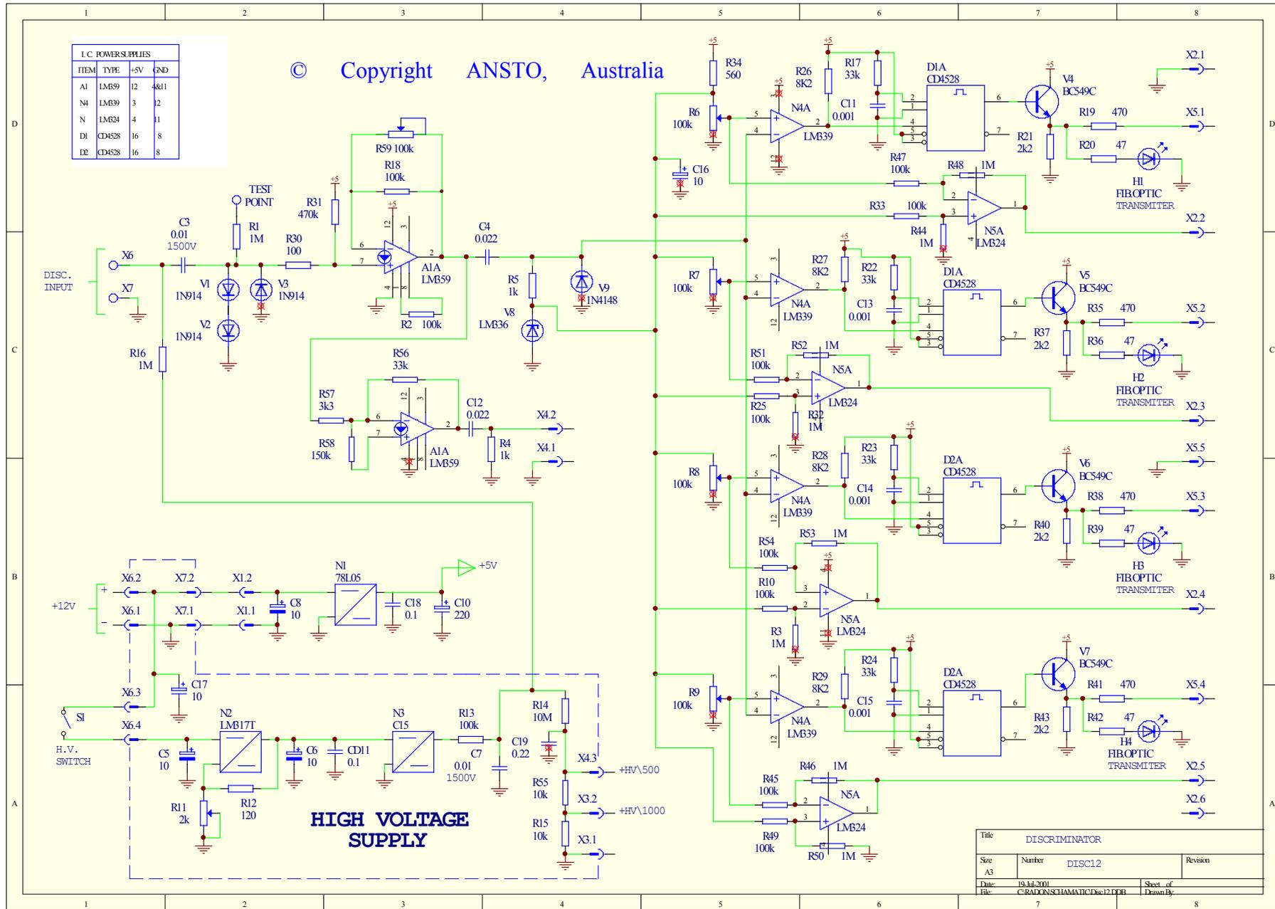
Figure 44: Schematic of the High Voltage/discriminator unit.
