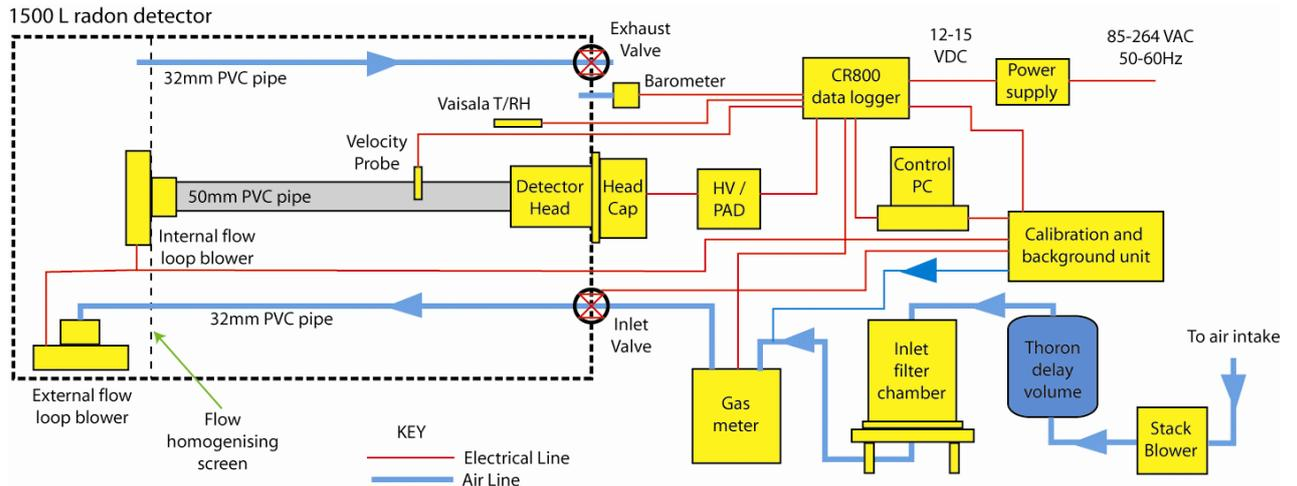
Figure 2: Schematic of an ANSTO two-filter detector setup similar to that installed at AIR-BOX.
