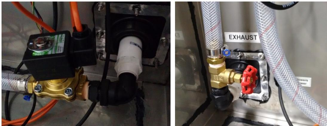
**Figure 7: (a) The inlet solenoid cut-off valve, and (b) exhaust line gate valve. These valves are located near the bottom of the electronics enclosure.**
