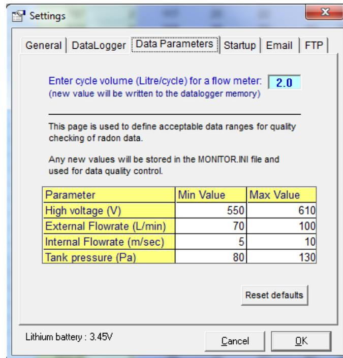
The radon detector is fitted with a gas meter that has been calibrated by the manufacturer. The gas meter's calibration constant (the "cyclic volume", expressed in litres per cycle) may vary depending on the model or manufacturer of the unit. The calibration constant is used to display the sampling flow rate correctly.
