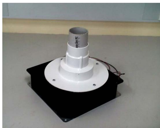
*Figure 10: Internal flow loop blower with 50mm PVC fittings.*
