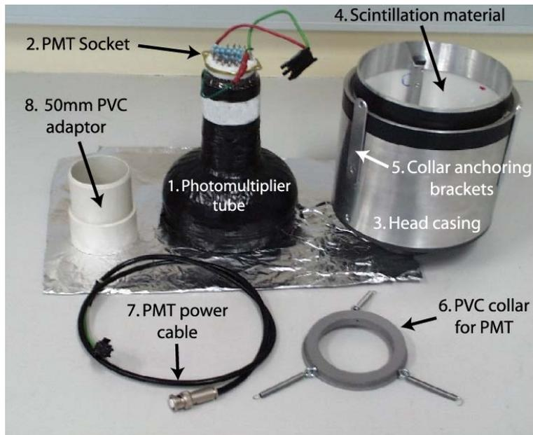
*Figure 20: Components of a radon detector head prior to assembly.*
