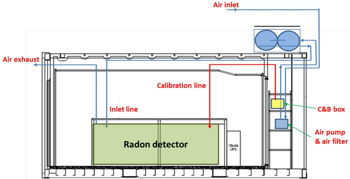
Figure 1: Location of radon detector in AIR-BOX container
