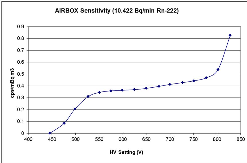
*Figure 36: Detector sensitivity as a function of high voltage setting onsite at AIR-BOX*
