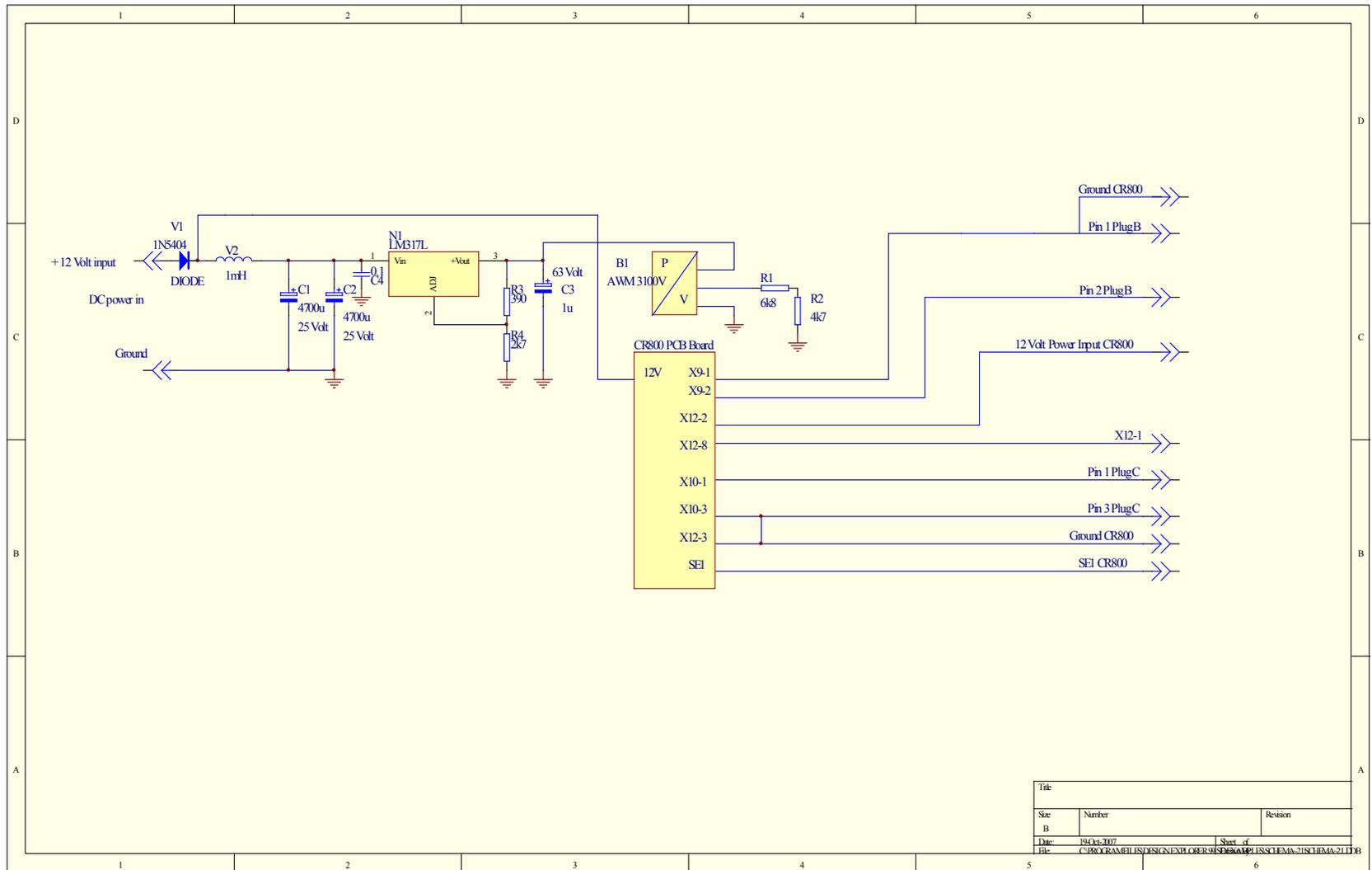
**Figure 43:** Schematic of the logger box integrated circuit board.
