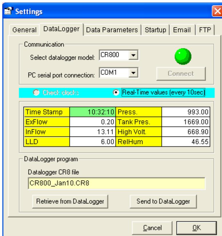
Once connected with the data logger, it is possible to display the 10-second average data of selected logger channels in real-time. Each time the data logger program executes, new values are written as input locations. These values are updated in the data logger every 10 seconds, as defined in the data logger program. This viewing
