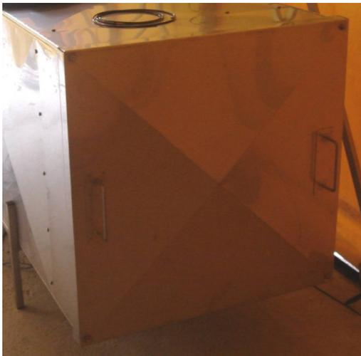
*Figure 12: Rear cover of the radon detector that provides access to the internal and external blowers.*
