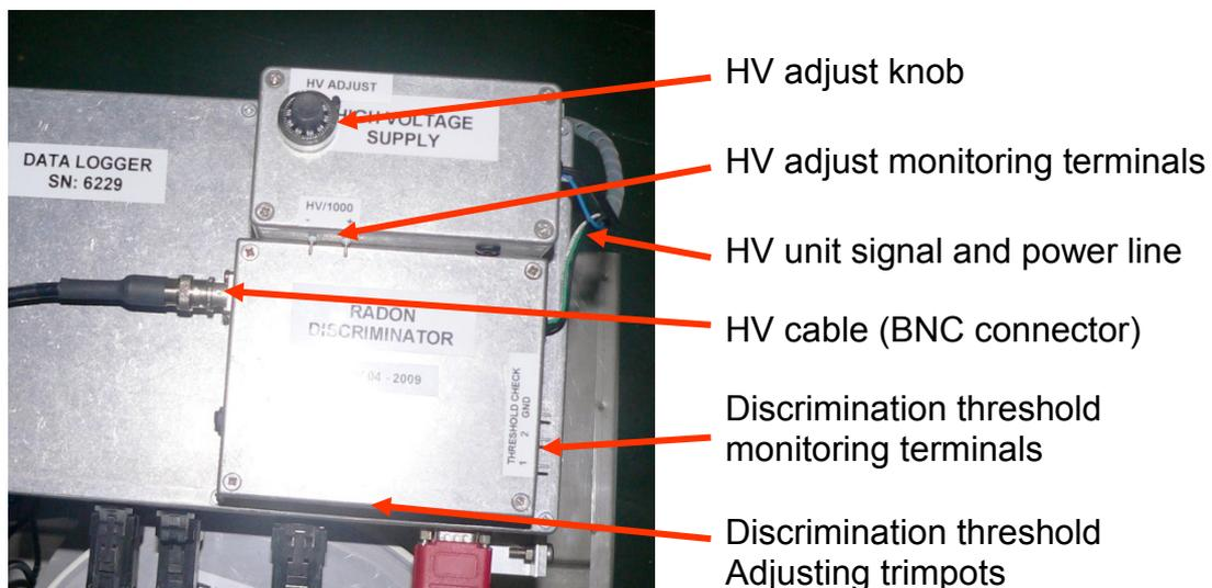
**Figure 25: High voltage / pre-amplifier, amplifier discriminator unit.**
