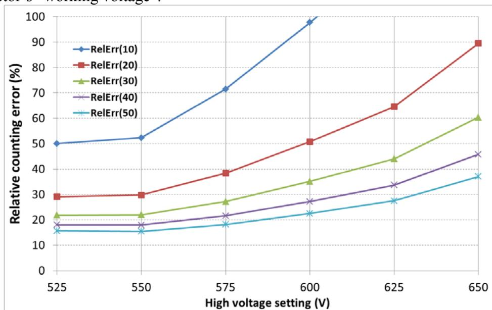
Figure 39: Relative error as a function of high voltage settings for a range of radon concentrations between 10 and 50  $\text{mBq m}^{-3}$  based on 2016 commissioning tests.
