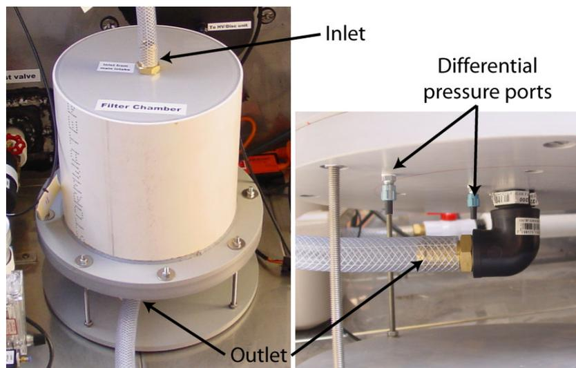
**Figure 15: Inlet filter chamber showing inlet, outlet and the differential pressure ports for monitoring the filter status.**
