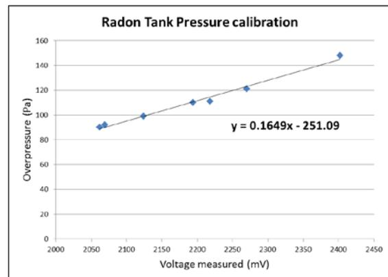
*Figure 28: Results of onsite pressure calibration performed and the linear approximation of the calibration curve.*
