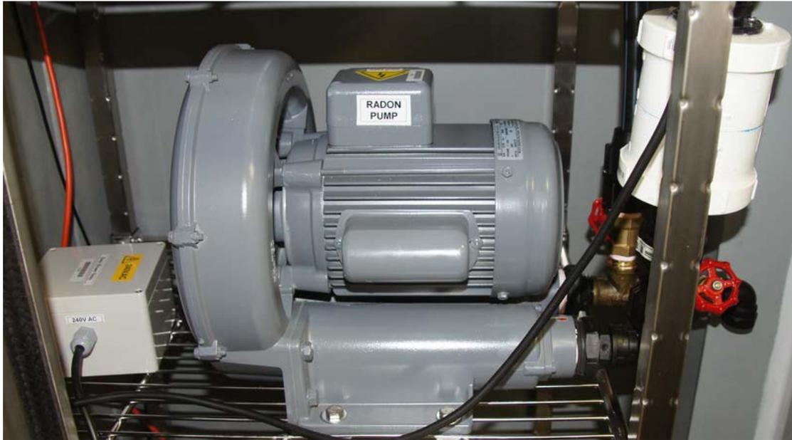
*Figure 4: Radon detector stack blower (240V;5A) and coarse air filter.*
