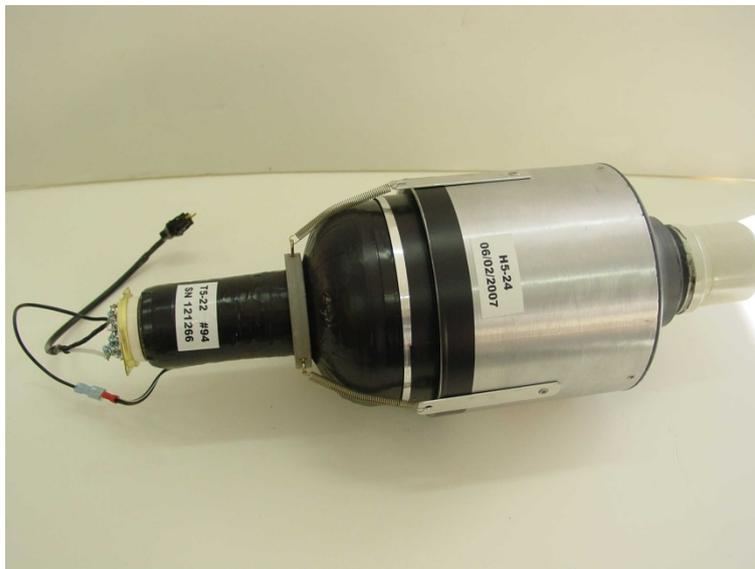
*Figure 21: Example of an assembled detector head ready for installation.*
