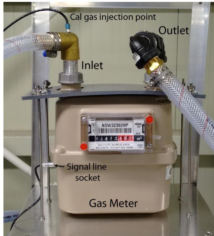
*Figure 16: Modified domestic gas meter used for monitoring the flow rate of the external flow loop; the leads from the internal optical counting device and the calibration gas injection port are shown.*
