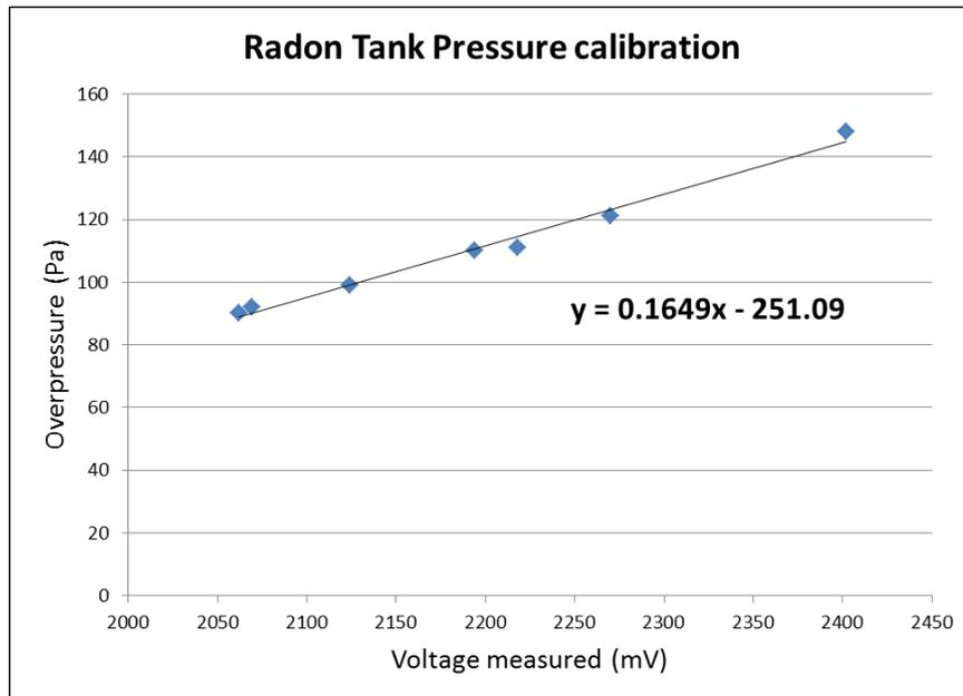
*Figure 8: Onsite tank pressure calibration*
