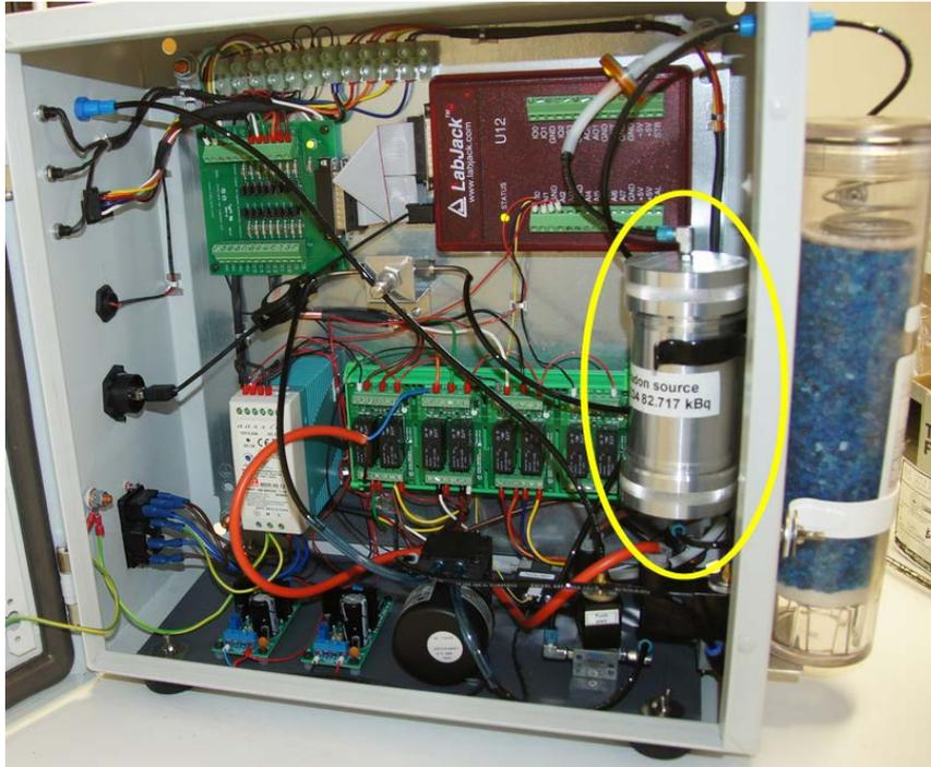
*Figure 35: Radon source inside the C&B unit.*
