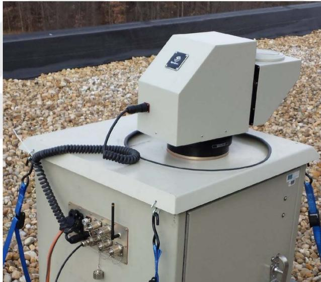
**Figure 4: MiniMPL Scanner Installed on Enclosure**
