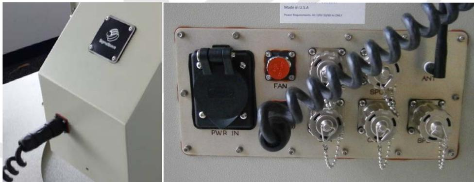
Figure 9: MiniMPL Scanner Cable Connections
